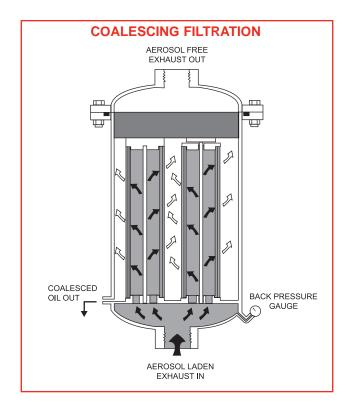
Headline CS-type Coalescing Filters are completely self-supporting and are sealed into the filter housing simply by tightening a retaining nut. No end caps, gasketing materials or support cores are required. At element change only the filtering material itself is discarded, and this complete disposability keeps replacement element costs down.
