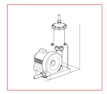
When vibration is excessive, or when temperature is high, or when cooling of the exhaust is desirable before coalescing, then the filter must be remotely mounted and connected by flexible ducting. The distance between the pump and the filter can be varied for convenience or to aid cooling, provided additional back pressure is not excessive.
